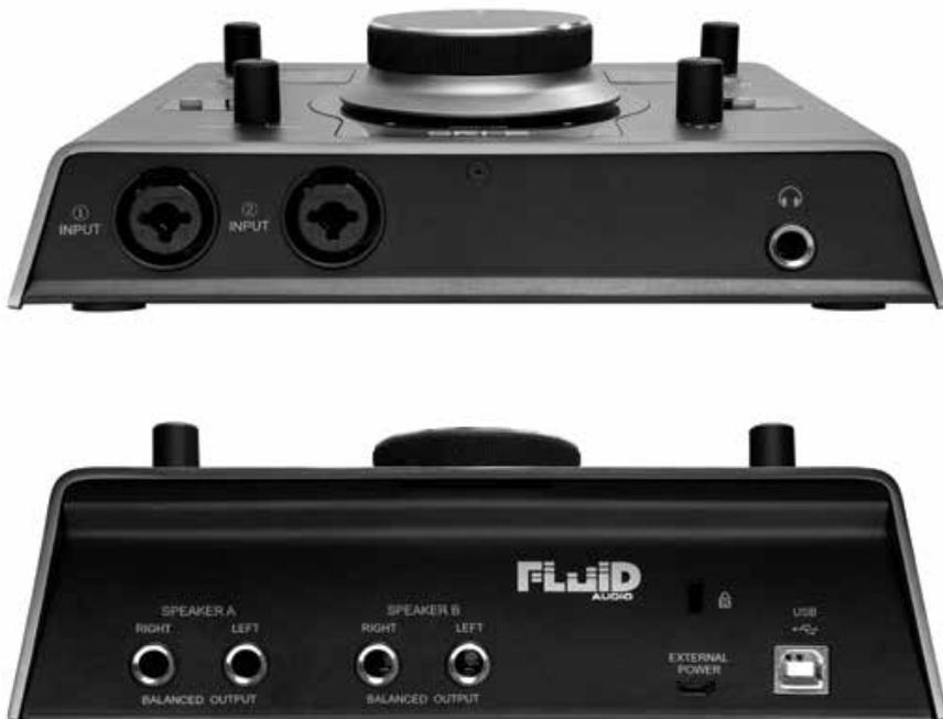
The inputs are conveniently placed on the front panel (top) with the speaker outputs on the rear panel (bottom)
