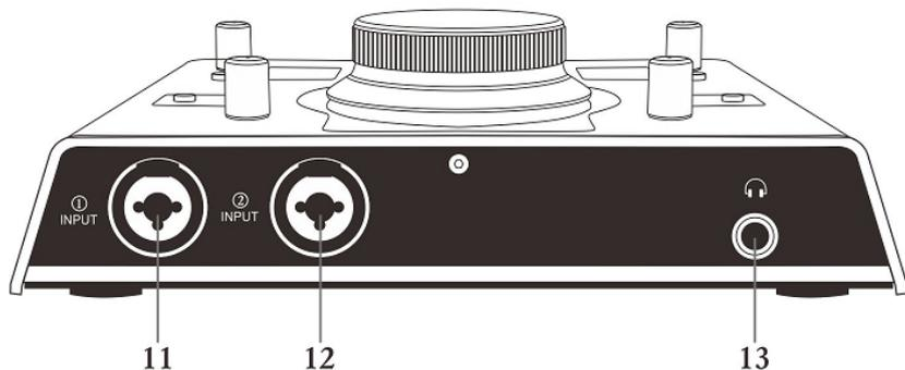
11. XLR/TRS Combo Input 1 (Mic/Line/Instrument)
